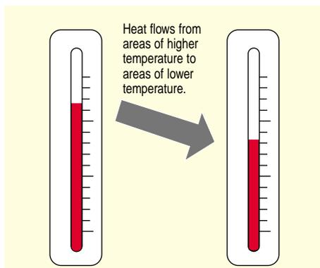
2. The greater the difference in temperature between two adjacent areas, the higher the rate of heat transfer between them.
